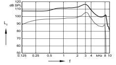
Output sound pressure level (L<sub>i</sub> = 90 dB)
