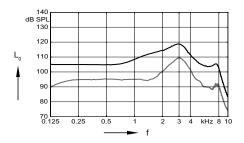
Max. Output sound pressure level (L<sub>i</sub> = 90 dB)
