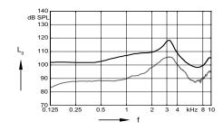
Max. Output sound pressure level (L = 90 dB)
