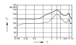
Max. Output sound pressure level (L = 90 dB)
