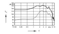
**Output sound** pressure level (L<sub>1</sub> = 90 dB)
