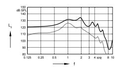
Max. Output sound pressure level (L<sub>i</sub> = 90 dB)
