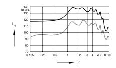
Max. Output sound pressure level (L<sub>i</sub> = 90 dB)
