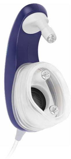
The spring-loaded electrodes adapt gently to any head-shape
