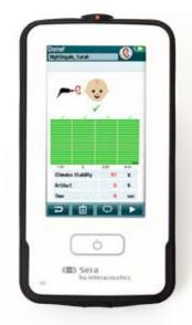
Sera™ offers fast DPOAE and TEOAE screening of newborn babies in an easy to use, handheld device. Place the probe in the baby's ear and a few seconds later clear test results will be displayed.
