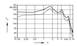
Max. Output sound pressure level (L<sub>1</sub> = 90 dB)
