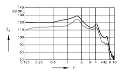
Max. Output sound pressure level  $(L_1 = 90 dB)$
